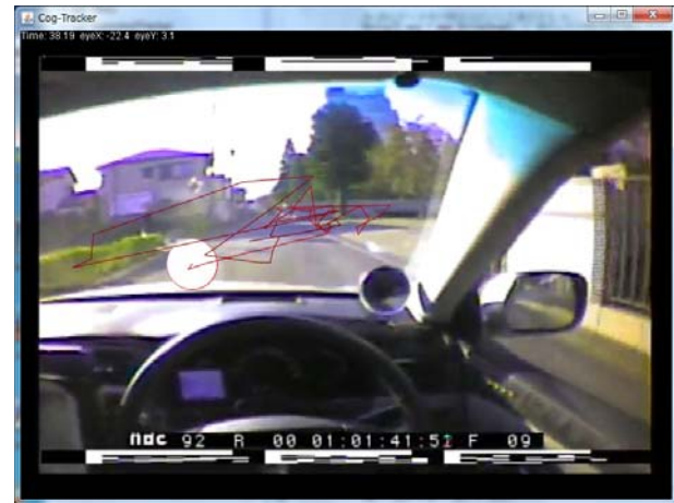
Figure 6: Visualization of eye movement over a certain period of time (5 sec. in the figure) presented by Cog-Tracker. The color becomes clearer as the visualization approaches the present time in the driving video
