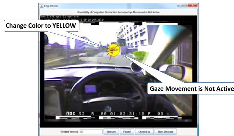
Figure 9: Detecting cognitive distraction using Cog-Tracker (2). Saccade frequency is reduced (no eye movement)
