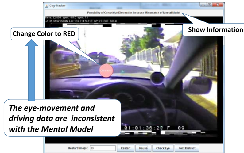
Figure 8: Detecting cognitive distraction using Cog-Tracker (1). The relationship between the eye movement and driving data was inconsistent with the mental model
