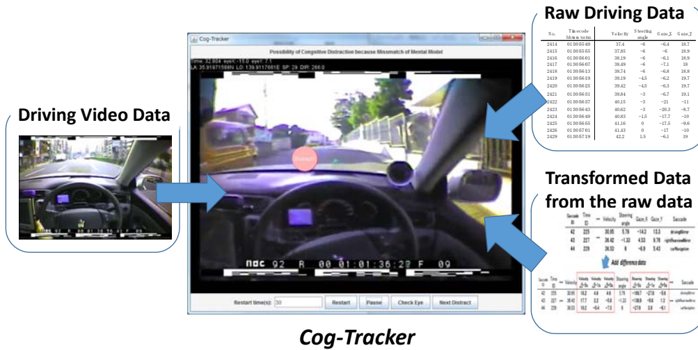
Figure 4: Cog-Tracker: This system extracts video driving data, raw data, and transformed data from the raw data. This is indicated by drawing a viewpoint circle at the current time during the driving video
