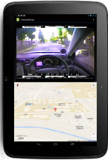
Figure 10: Cog-Tracker implementation on a tablet PC. This system can display video and map information to drivers
