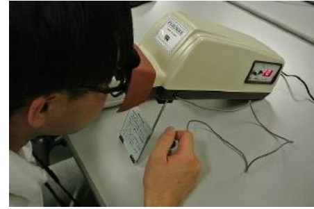
Figure 5: Experimental image of measuring CFF value
