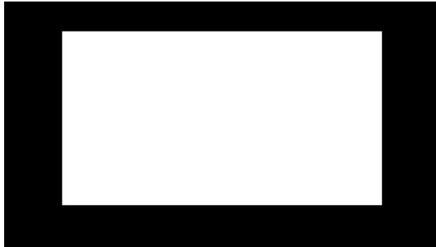
Figure 4: The source image used for projector-camera homography calculation. The image dimensions are 1920 by 1080 pixel
