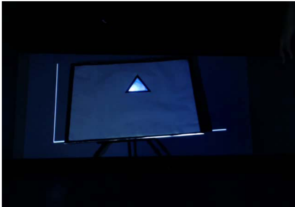
Figure 14: Triangular ROI is introduced over the planar surface. The system identifies the shape and projects over it, while it moves in the planar surface
