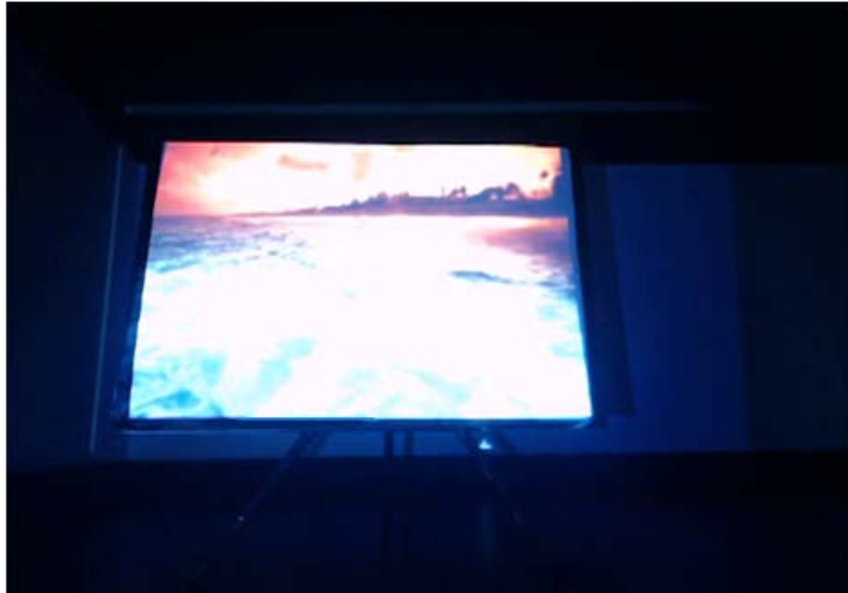
Figure 12: Planar surface is used a display screen, while ROI is not provided. The projection is keystone corrected and does not bleed out of the planar surface
