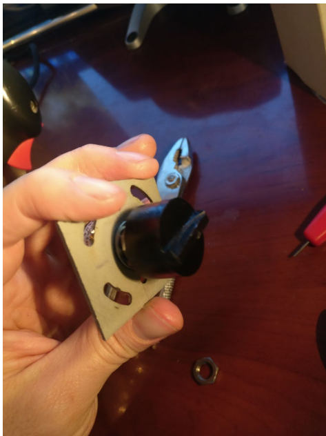
Figure 8: The potentiometer inside the joystick x-axis. The potentiometer senses the axis position and conveys the information over 3 voltage regulated wires
