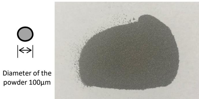
Figure 12: Stainless steel particle
