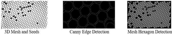
Figure 3: Mesh detection using pixel color
